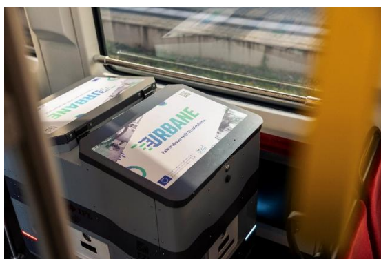
FIGURE 16: DELIVERY ROBOT IN MULTIPURPOSE SPACE WITHIN TRAM – HIGH MANEUVERABILITY BY OMNIDIRECTIONAL CHASSIS (HERE: LATERAL DRIVING)
