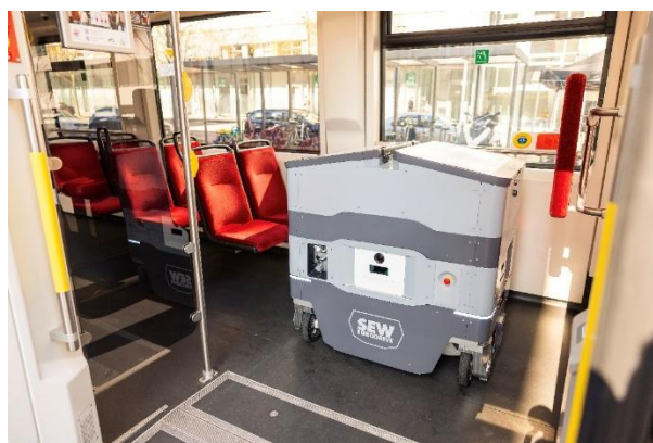
FIGURE 16: DELIVERY ROBOT IN MULTIPURPOSE SPACE WITHIN TRAM – HIGH MANEUVERABILITY BY OMNIDIRECTIONAL CHASSIS (HERE: LATERAL DRIVING)
